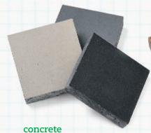
WHAT IT IS: Cement, water, sand, stone, and pigment formed into a slab. PROS: "The surface is incredibly smooth," says Paula Flanagan, an interior designer in Chicago. And it's customizable. Tint it to match a paint color, embed it with shells, and choose any thickness.
